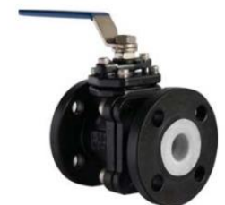
PLASTIC LINED 2 piece - Full Port ANSI 150 (DN15 - DN100) PN10 (DN50 - DN200)
